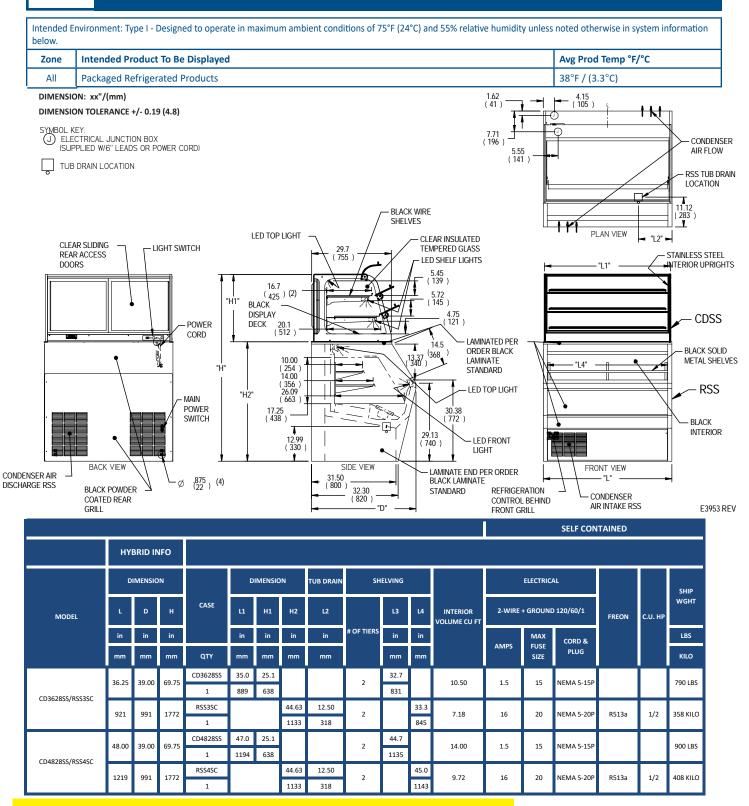
× On the RSS6SC a separate 120/60/1 15 AMP circuit is required for the condensate evaporator.
