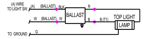
(SEE MAIN WIRING DIAGRAM DETAIL)
