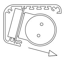
6. Reinstall new bulb in the same manner as described in the Bulb Removal Procedure. Be sure bulb is secure in bulb receptacles.
