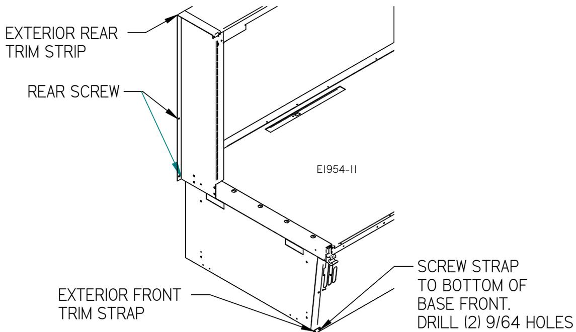
2. Remove the adhesive liner from the inside of the rear exterior trim strip and firmly place it over the top and down the back of case. Be sure to center rear exterior trim strip over seam between cases and to align slots with holes in case rear (If holes are provided)
