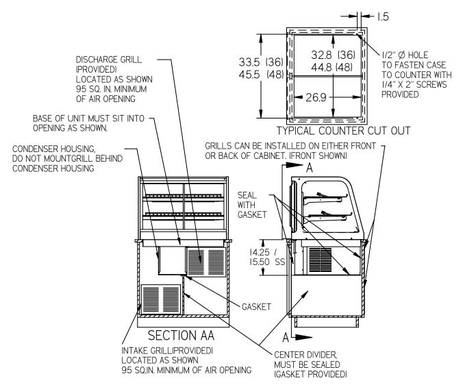
**CORD OPTION 1:** The electrical cord is shipped from the factory protruding from the bottom rear corner of the base and will fall through the required cut in counter. After the case has been installed and fastened onto the counter, plug cord into a proper power source.
