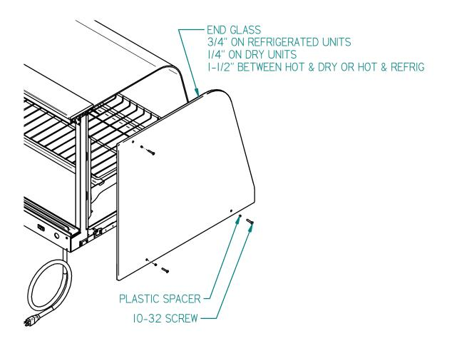
End panels are Ordinarily shipped loose from the factory and need to be installed once the case fastened to the counter. When placing cases in a line up the number of end panels and end panel type will be different for each line up circumstance. See Case Line Up Installation section of this manual.
