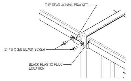
All cases joined together should have a top joining bracket installed to keep the top of the case tight together. There are different brackets included with each case to cover most joining combination needs. If no holes are provided, drill a 1/8" dia x  $\frac{1}{2}$ " deep hole in location needed for bracket attachment.
