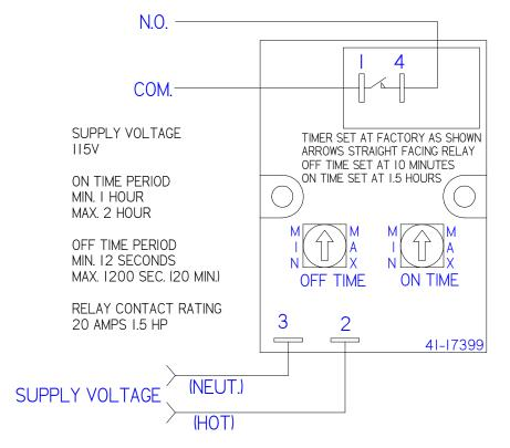
OPERATION: APPLY SUPPLY VOLTAGE - RELAY TRANSFERS ICONTACT CLOSES) AND TIME PERIOD I (ON TIME) BEGINS. AFTER INITIAL DELAY, RELAY TRANSFERS AGAIN (CONTACT OPENS) FOR DURATION OF TIME PERIOD 2 (OFF TIME) THIS RECYCLING CONTINUES UNTIL SUPPLY VOLTAGE IS REMOVED
