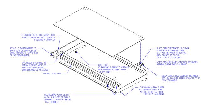
1. For first time installation attach (2) glass shelf holders to each glass shelf. Remove backing from tape located on flat side of glass shelf holder. Position the glass shelf holders in the (2) far corners of glass. Repeat for each glass shelf. Attach a clear bumper on both sides of the light housing top surface for the front of the glass to set on. This step may have already been performed at the factory for you.
