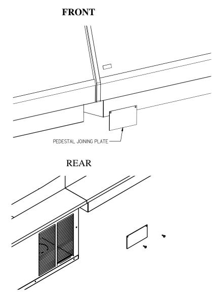
The CRR model cases and cases with optional pedestal have a 2-3/4" pedestal that sets on top the counter. When these cases are joined there is a gap between the pedestals. Two joining plates are provided for these models.
