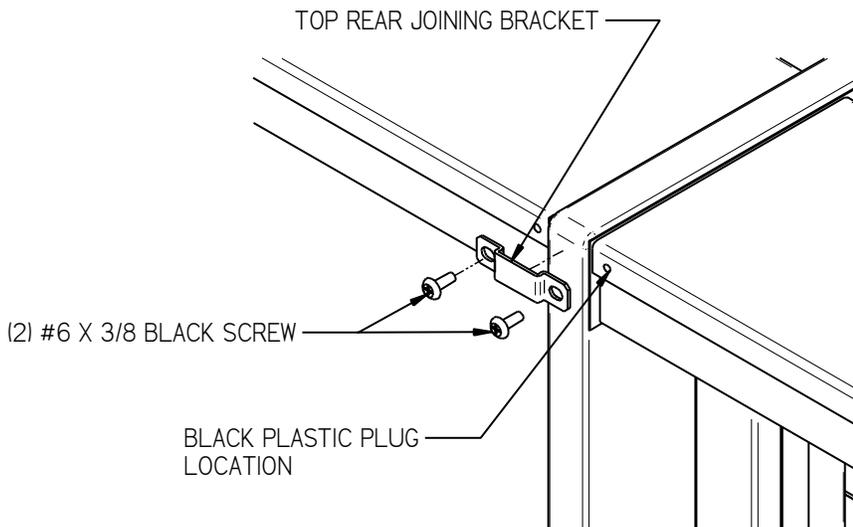
All cases joined together should have a top joining bracket installed to keep the top of the case tight together. There are different brackets included with each case to cover most joining combination needs. If no holes are provided, drill a 1/8" dia x 1/2" deep hole in location needed for bracket attachment.
