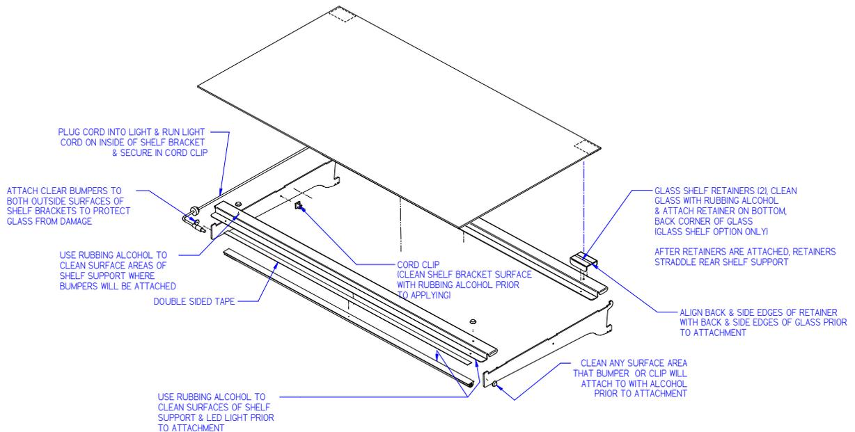
1. For first time installation attach (2) glass shelf holders to each glass shelf. Remove backing from tape located on flat side of glass shelf holder. Position the glass shelf holders in the (2) far corners of glass. Repeat for each glass shelf. Attach a clear bumper on both sides of the light housing top surface for the front of the glass to set on. This step may have already been performed at the factory for you.
