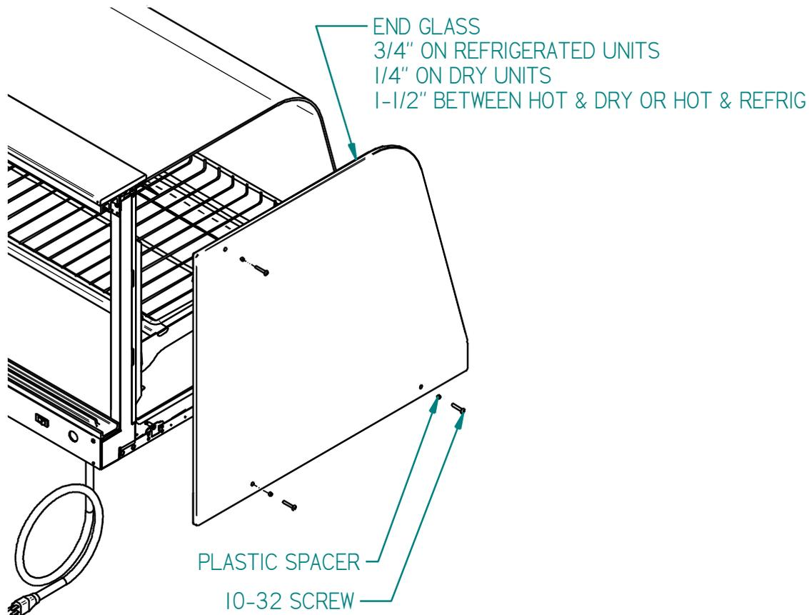
End panels are Ordinarily shipped loose from the factory and need to be installed once the case fastened to the counter. When placing cases in a line up the number of end panels and end panel type will be different for each line up circumstance. See Case Line Up Installation section of this manual.
