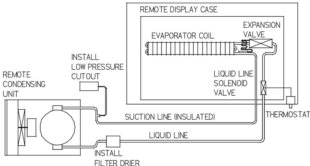
1. Mount condensing unit indoors as close to the remote display case as practical. The refrigeration line should be as short as possible and must not exceed 30 feet.
