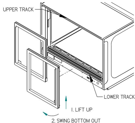
1. Start with the outer door and lift the door upward until the bottom edge of door clears the lower track and then swing the bottom of the door outward and down out of upper track.
