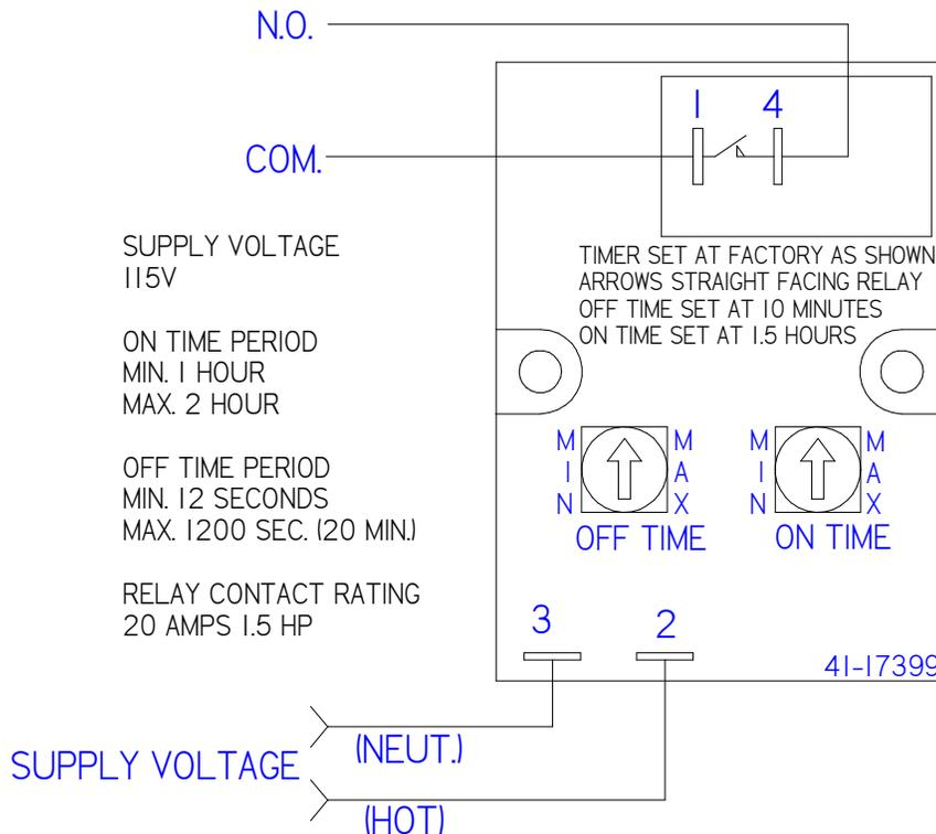
OPERATION: APPLY SUPPLY VOLTAGE - RELAY TRANSFERS (CONTACT CLOSES) AND TIME PERIOD 1 (ON TIME) BEGINS. AFTER INITIAL DELAY, RELAY TRANSFERS AGAIN (CONTACT OPENS) FOR DURATION OF TIME PERIOD 2 (OFF TIME) THIS RECYCLING CONTINUES UNTIL SUPPLY VOLTAGE IS REMOVED
