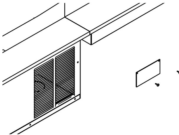
The CRR model cases and cases with optional pedestal have a 2-3/4" pedestal that sets on top the counter. When these cases are joined there is a gap between the pedestals. Two joining plates are provided for these models.
