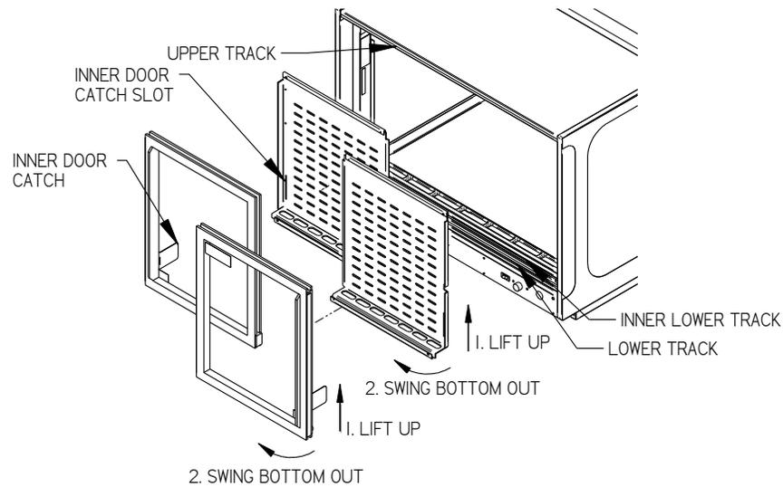
1. Start with the outer outside door and lift the door upward until the bottom edge of door clears the lower track and then swing the bottom of the door outward and down out of upper track.
