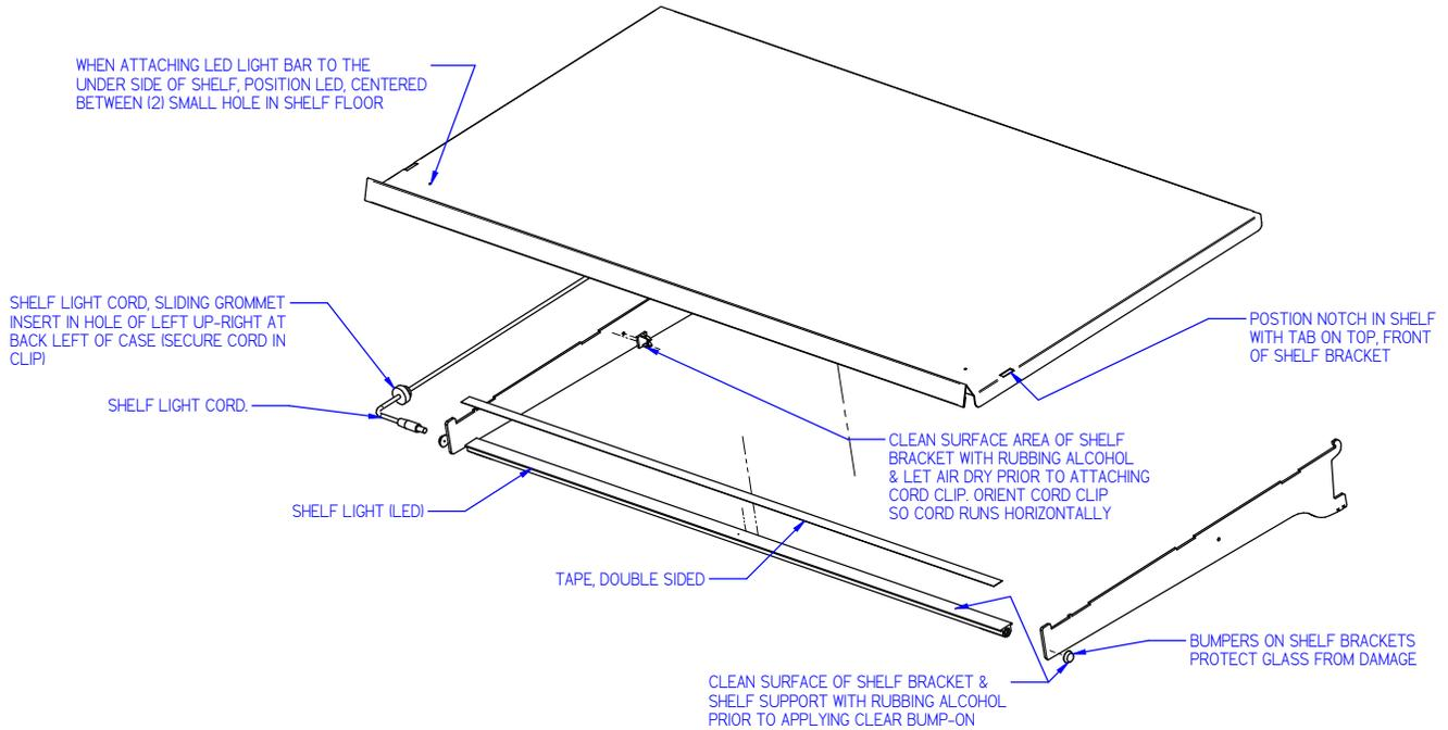
1. With rear sliding doors removed, place front of the metal shelf onto front shelf light. (On front shelf support for models without shelf lights)
