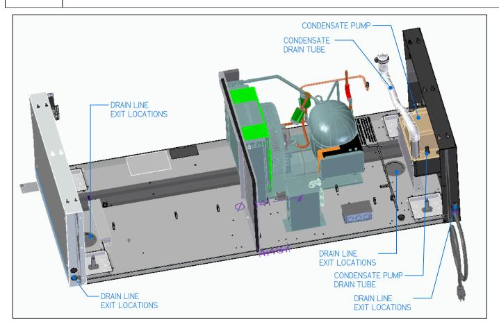
Instead of using heat energy to remove condensate run off from the evaporator coil a condensate pump moves the water to a nearby drain.
