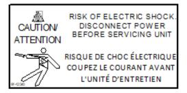
This label is located behind the removable base deck panels display and under deck pans.
