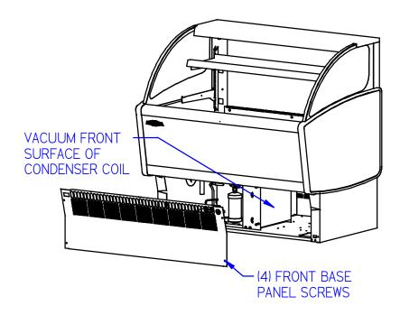
Figure 1 - Condenser Cleaning
