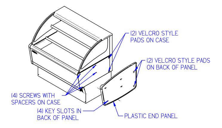
Right and Left plastic end panels are ordinarily shipped installed from the factory but can be easily removed for cleaning. Removing end panels make it easier to grab on to case when moving or installing case and can easily be reinstalled.
