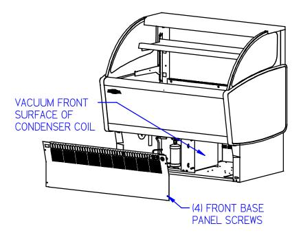
Figure 1 - Condenser Cleaning
