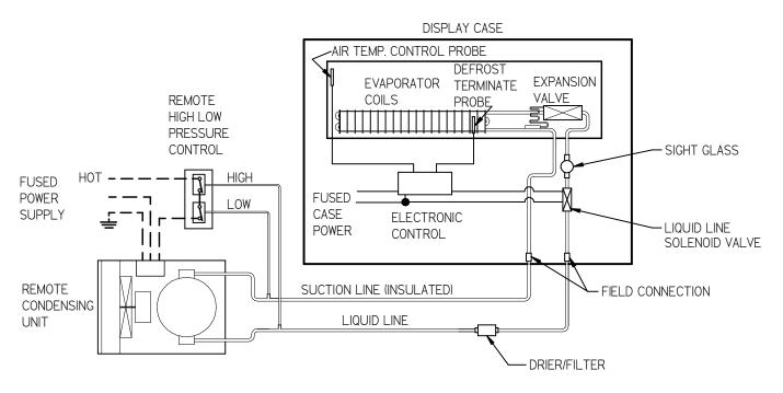
Figure 2 - Remote Refrigeration Diagram
