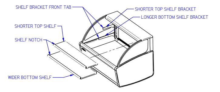
1. Follow the instructions in the illustration below and insert (1) of the shelf brackets in the desired shelf standard slot on one side of the case. Place the additional bracket in the same shelf standard slot on the opposite end of case. If the case was supplied with shelf light option (ELPRSS), the bracket with a clear plastic cord retainer clip must be on the side with the shelf light. For LPRSS case with (2) shelves repeat for shorter top shelf brackets.
