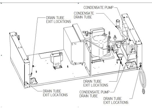
Instead of using heat energy to remove condensate run off from the evaporator coil a condensate pump moves the water to a nearby drain.
