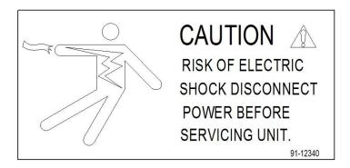
Before any service work is performed on the case, make sure all power is disconnected to the case.
