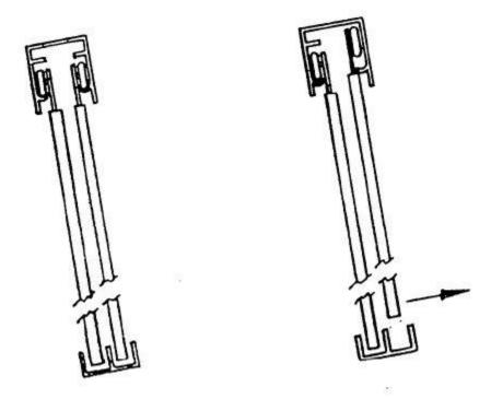
To remove the door closing spring, grasp the spring several inches from the end and slip the spring end loop off the clip located in the upper channel.
