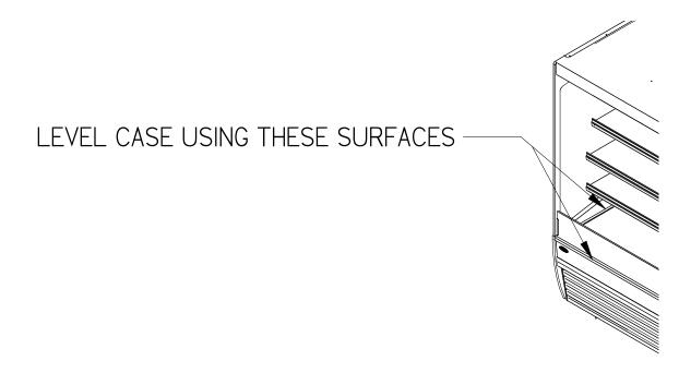
Adjust the (4) outside leg levelers as needed to level the case in each direction.
