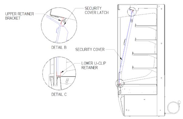
When installing the security cover panel, ensure that the bottom of the panel is seated in the lower u-clip, and that the latch fully engages behind the upper retaining bracket.
