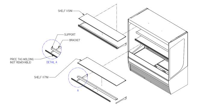
The diagram below illustrates how to straighten or angle the shelves. To angle the bracket, be sure to have the top hook of the bracket in its slot and to pull up while rotating down to the most extreme downward position. To angle the shelf, first angle both brackets, and install the shelf as normal.
