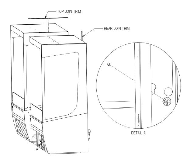
7. Finish the joining process loosening the glass trim on the case to slide the joining trim over the existing trim and secure with the existing fasteners. Do this for both the top trim and the rear trim.
