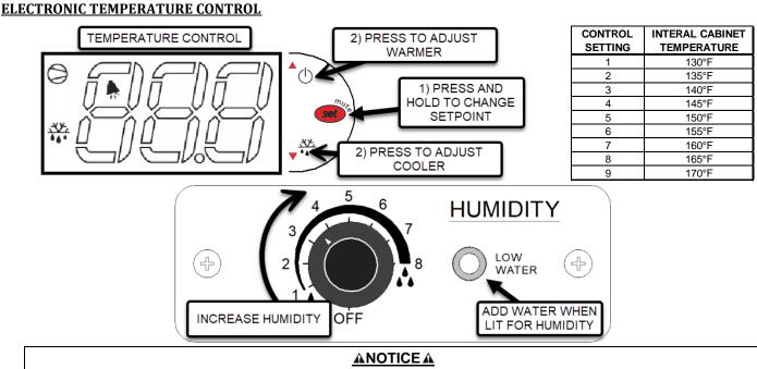
This heated display case is designed to operate in an environment of 70°F. Temperatures less than this may cause performance issues.
