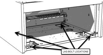
Once all the bolts are removed, slide the unit off the back of the shipping pallet, and tilt it so the rear corner touches the ground. Then have someone move pallet out from under the case and gently tilt the case forward until it touches the floor. Shelves, doors, and front glass may be removed from the unit to reduce overall weight.
