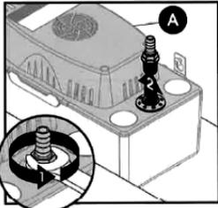
If equipped, check that condensate pan or pump is properly plugged in or hardwired to power. If the pump is running, but cannot evacuate to water, clean the condensate pump impeller, drain tube and discharge tubing or replace pump assembly as required.
