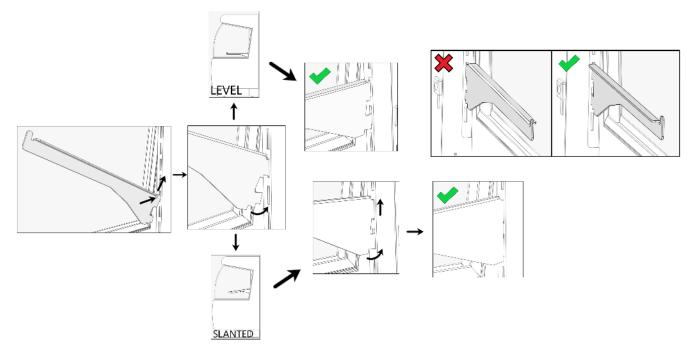
Lay back of shelf across both brackets. Slide it to the rear and then lay the front of the shelf down. Check that the retaining tab of the shelf brackets protrudes through the slot in the shelf.
