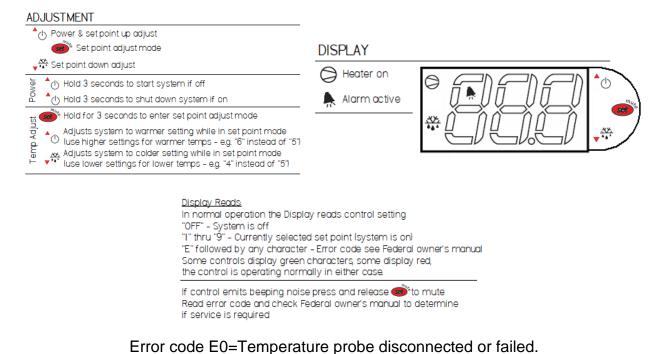
The temperature controllers each reference one temperature probe that is mounted in the deck or shelf depending on the control. Do not locate the probe to a different position.
