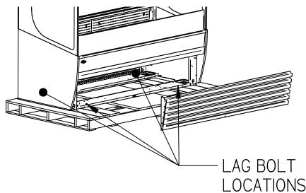
Once all the bolts are removed, slide the unit off the back of the shipping pallet, and tilt it so the rear corner touches the ground. Then have someone move pallet out from under the case and gently tilt the case forward until it touches the floor.
