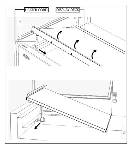
To remove the deck simply lift on the front handle and rotate the front of the deck upward. Hold the assembly in place and use your other hand to disengage the heater cord from the tub. Then simply lift the deck from the unit. Installation is the reverse of removal.
