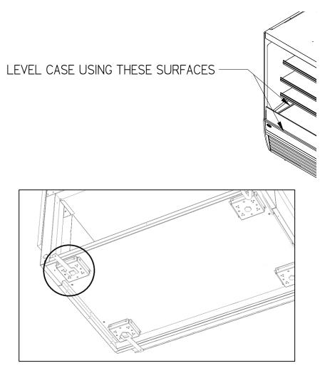
Adjust the (4) outside leg levelers as needed to level the case in each direction.
