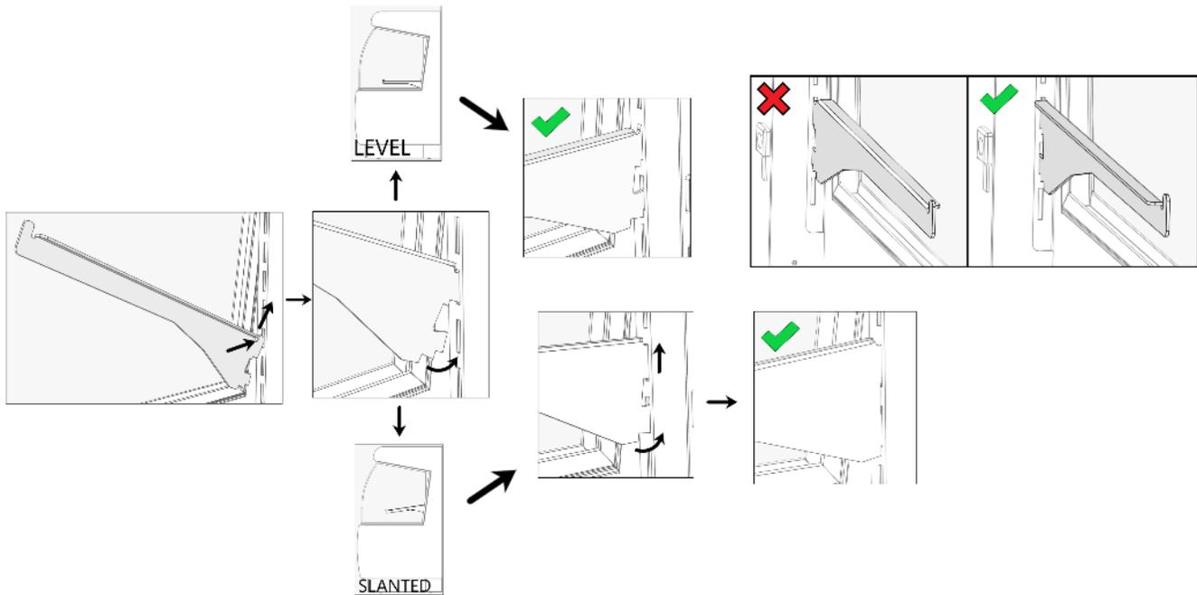
Lay back of shelf across both brackets. Slide it to the rear and then lay the front of the shelf down. Check that the retaining tab of the shelf brackets protrudes through the slot in the shelf.
