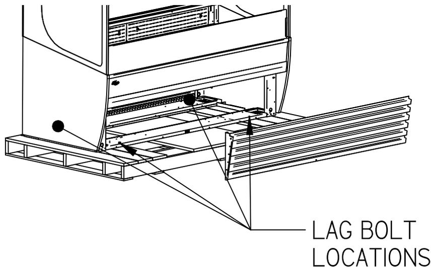
Once all the bolts are removed, slide the unit off the back of the shipping pallet, and tilt it so the rear corner touches the ground. Then have someone move pallet out from under the case and gently tilt the case forward until it touches the floor.
