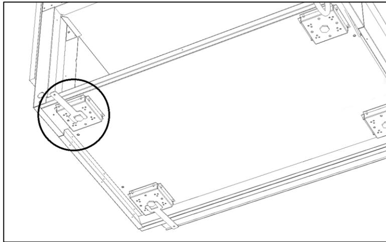
Adjust the (4) outside leg levelers as needed to level the case in each direction.
