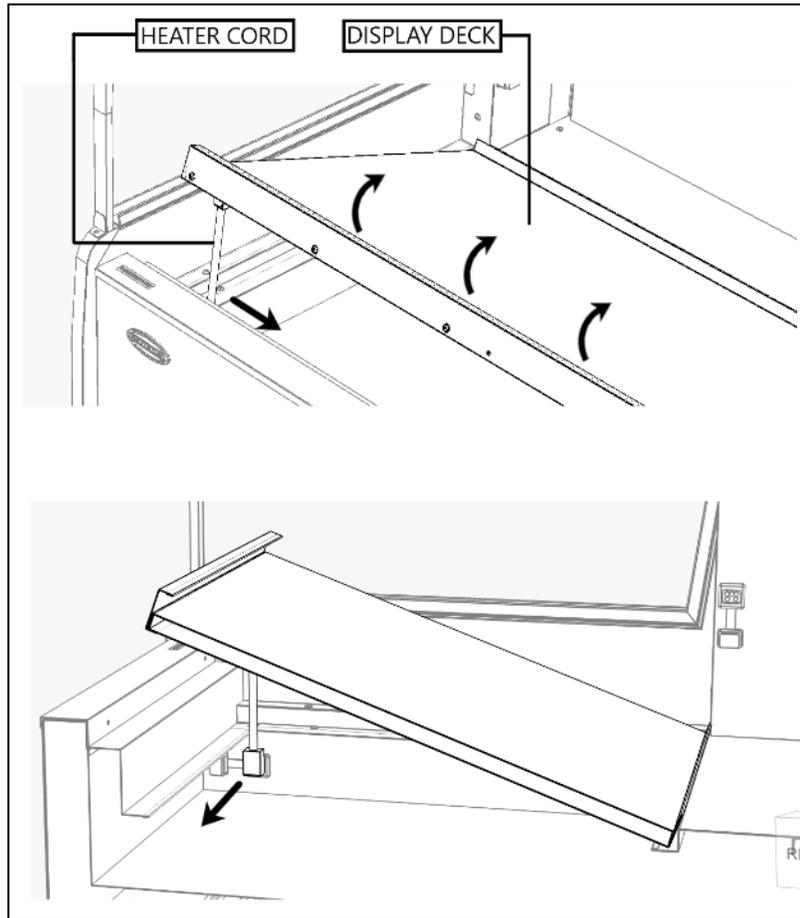
To remove the deck simply lift on the front handle and rotate the front of the deck upward. Hold the assembly in place and use your other hand to disengage the heater cord from the tub. Then simply lift the deck from the unit. Installation is the reverse of removal.
