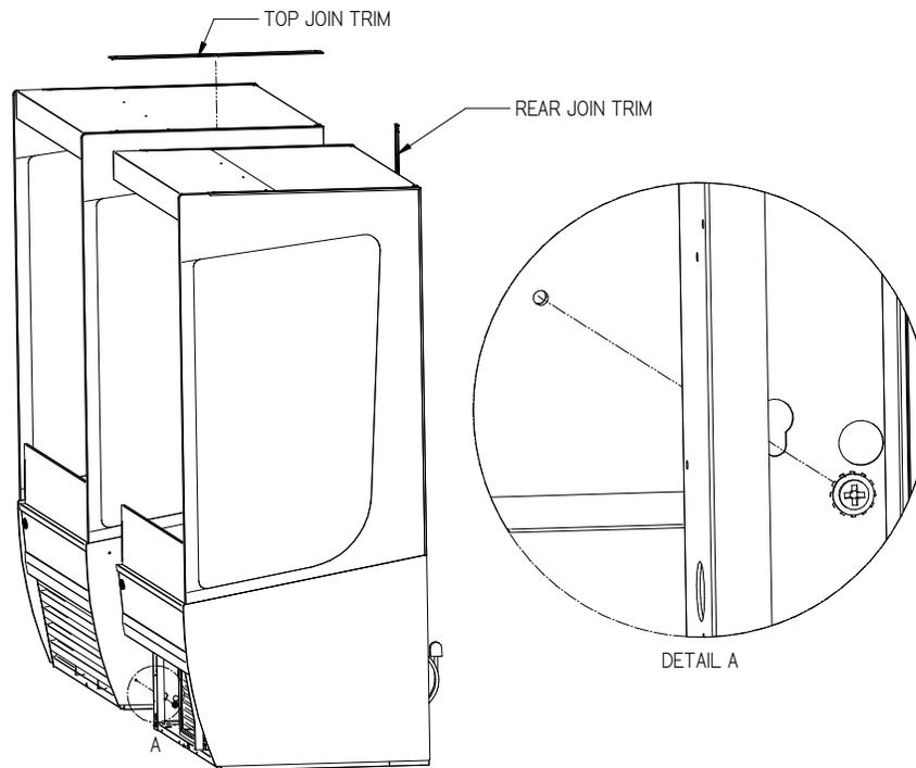
7. Finish the joining process loosening the glass trim on the case to slide the joining trim over the existing trim and secure with the existing fasteners. Do this for both the top trim and the rear trim.
